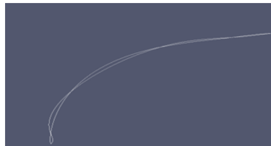
Figure 3: Schematic showing an exaggerated effect of the geometry oscillations in a very coarse curved edge.
