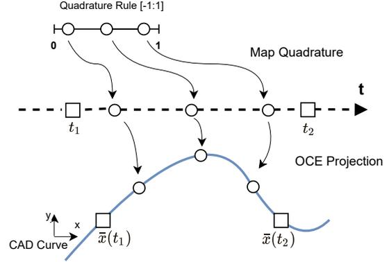
**Figure 5:** Parametric projection for an edge with a single CAD curve.
