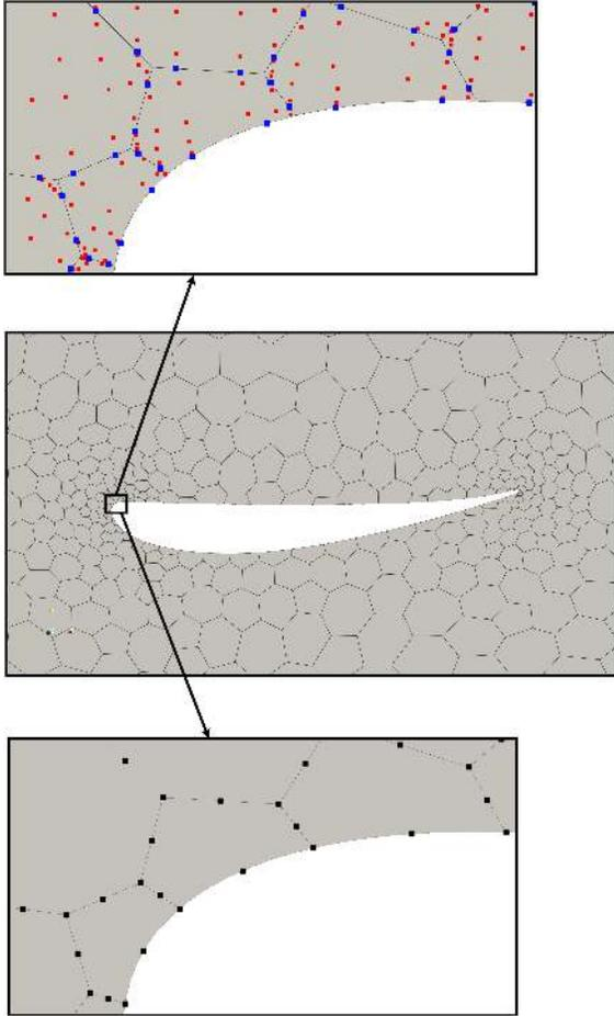
**Figure 14:** A curvilinear high-order polygonal mesh of an automotive aerofoil. The mesh of the domain only displays the edges of the polygonal elements. An enlargement of the mesh near the boundary illustrates the additional degrees-of-freedom required for the high-order discretization. The top window shows the locations of the quadrature points on the edges (blue) and on the interior (red) of the polygonal cells. The bottom window shows the locations of the points used for interpolation.
