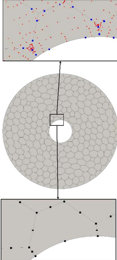
**Figure 10:** A curvilinear high-order polygonal mesh of the domain  $\Omega$ . The mesh of the domain only displays the edges of the polygonal elements. An enlargement of the mesh near the boundary illustrates the additional degrees-of-freedom required for the high-order discretization. The top window shows the locations of the quadrature points on the edges (blue) and on the interior (red) of the polygonal cells. The bottom window shows the locations of the points used for interpolation.
