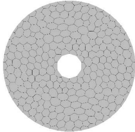
**Figure 4:** A coarse uniform linear mesh of a ring with interior radius  $R_1 = 0.2$  and exterior radius  $R_2 = 1$ .
