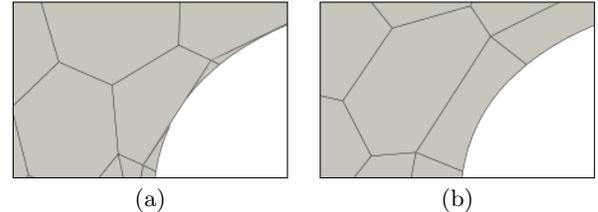
**Figure 7:** A mesh with a layer of stretched quadrilaterals: (a) A layer thickness below the value  $\delta_{\min}$  given by equation (5) leads to self-intersection and thus invalid elements; (b) A valid mesh is obtained with a value above the minimum thickness.
