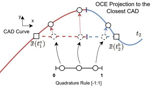
**Figure 6:** Projection for a straight edge with 2 CAD curves.
