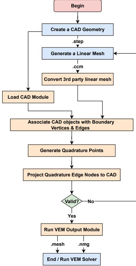
**Figure 8:** The workflow of the proposed pipeline from the CAD definition to the curvilinear high-order mesh.
