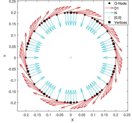
**Figure 9:** Visualization of the high-order geometrical information (with  $k = 2$ ) communicated to the VEM solver via the `.nmg` file.
