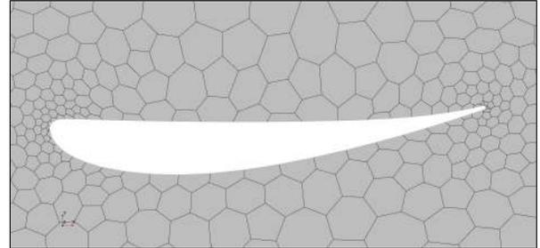
**Figure 13:** A straight-sided linear mesh of an automotive aerofoil.
