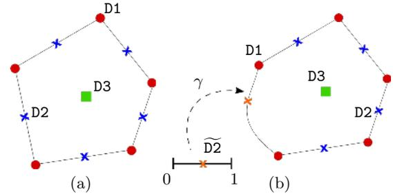
**Figure 1:** Degrees of freedom for the straight case (a) and for the curved case (b) with polynomial order  $k = 2$ . The mapping  $\gamma(t)$  ( $0 \leq t \leq 1$ ) is used to define the curved edge.
