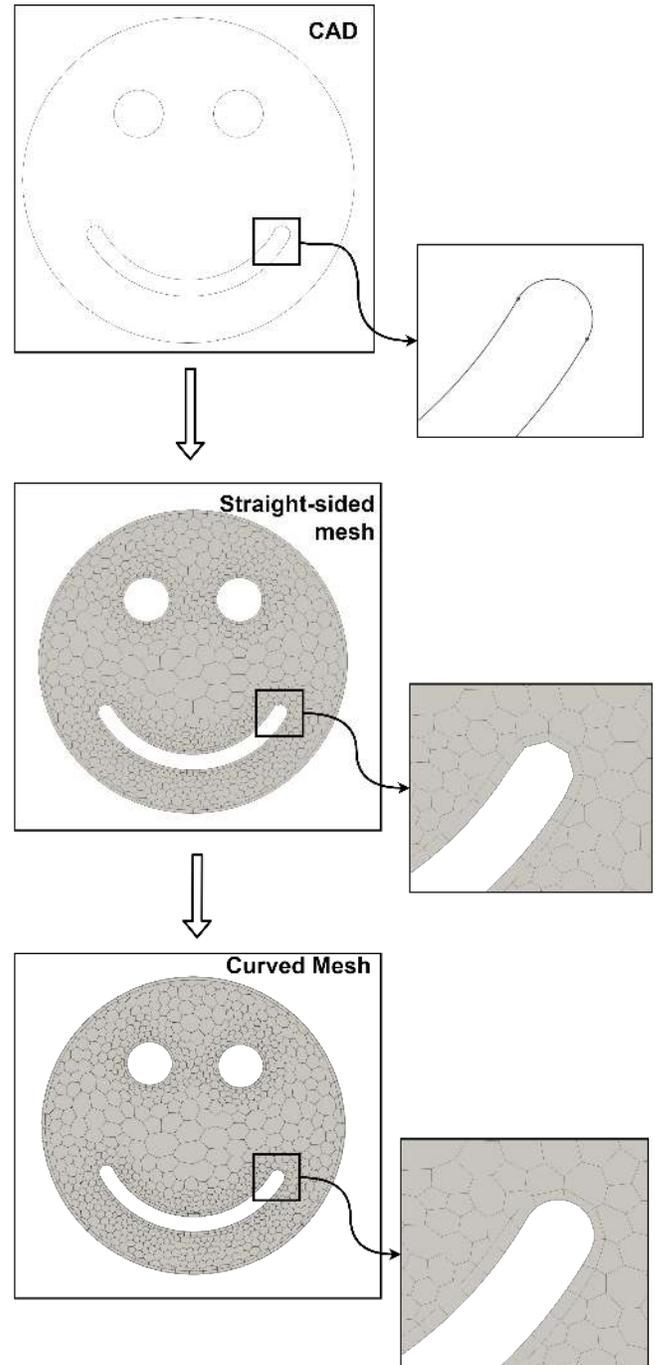
**Figure 3:** The *a posteriori* approach to high-order VEM mesh generation. From top to bottom: CAD B-Rep definition of the domain, straight-sided polygonal mesh, and curvilinear high-order mesh.
