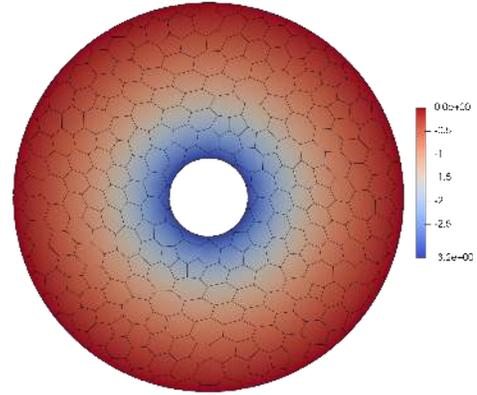
**Figure 12:** High-order VEM solution ( $k = 2$ ) of the Laplace equation with Dirichlet boundary conditions computed on a curvilinear mesh (`withGeo`).
