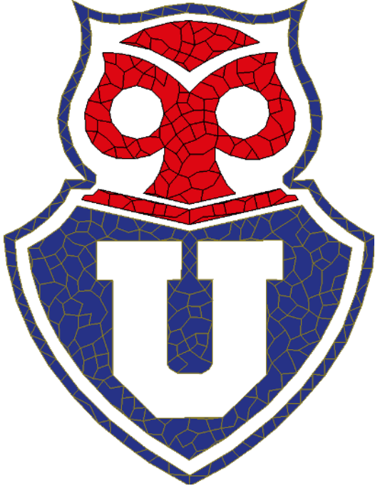
Figure 1: Polylla mesh of the football team Club Universidad de Chile’s logo. The mesh contains 410 polygons and 1039 edges. White spaces represent holes.
