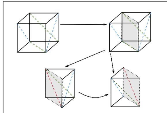
**Figure 7:** Decomposition of a single pair with different orientations: (*Top*) The side opposite to the green cut is chosen so that two of the predetermined cuts get isolated in one of the prisms. (*Bottom-Left*) The red diagonal is chosen to configure the prism to **FFR**. (*Bottom-Right*) The green cut is then picked to avoid the degenerate cases.
