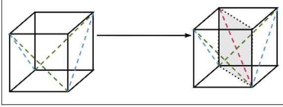
**Figure 8:** Decomposition of both pairs meeting at a vertex with different orientations: This ensures that we have a pair of opposite uncut faces. (Right) Consequently, we can decompose into prisms and choose the red diagonal cut to avoid the degenerate case.
