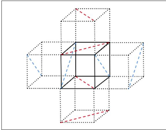
**Figure 11:** Degenerate case for cubes when flipping opposite face cuts of adjacent cubes: This is an instance when flipping fails as all four adjacent cubes' opposite faces have cuts with different orientations.
