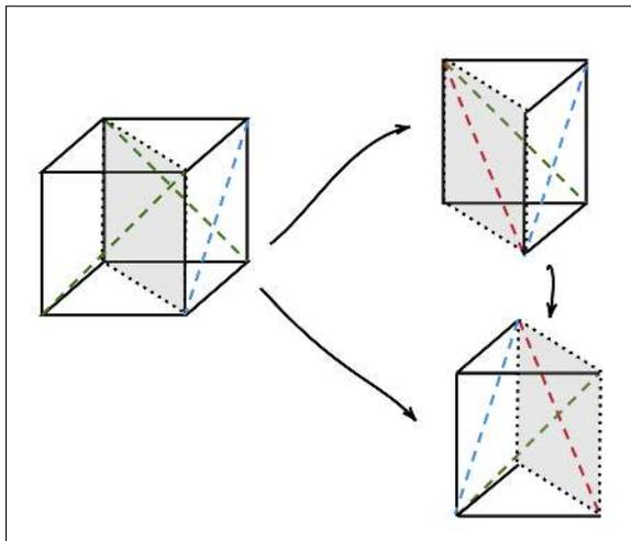
**Figure 6:** Three predetermined cuts: two of the three cuts form a pair with opposite orientation. (*Left*) We first choose a dividing plane. (*Upper-Right*) Then, the red diagonal is chosen to configure the prism with two external predetermined cuts to **FFR**. (*Lower-Right*) Finally, the blue cut is then picked in the second prism to avoid the degenerate cases.
