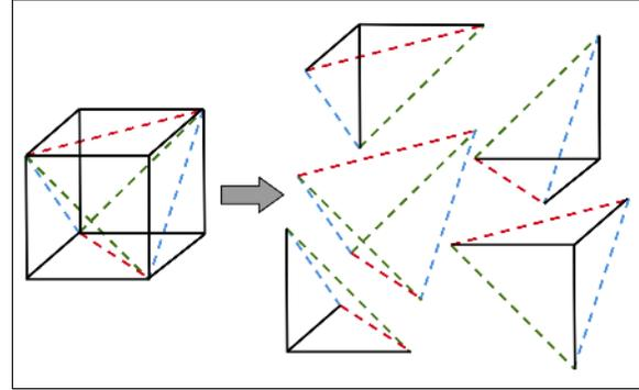
**Figure 10:** The five tetrahedral decomposition: (Right) An implementation of this decomposition can be done by simply removing the central tetrahedron; the rest of the four tetrahedra are distributed along the four corners.
