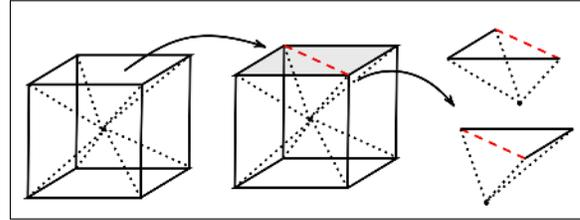
**Figure 12:** Steiner points allows decomposition into twelve tetrahedra at the expense of an additional vertex: (Left) We first connect each of the vertices with the Steiner point. (Middle, Right) This yields six pyramids, which is then cut across to get tetrahedra using the predetermined cuts (red).
