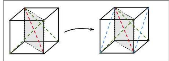
**Figure 5:** Two predetermined cuts (green): cutting with the opposite faces in the same orientation (blue) yields **FFR** for both prisms.
