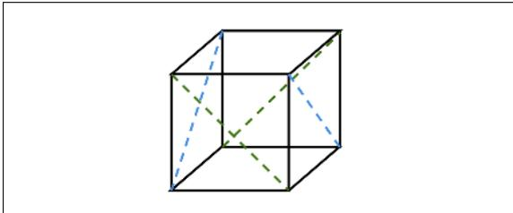
**Figure 9:** Degenerate case for a cube with four determined cuts. The case for degenerate case for cubes with more than four determined cuts is omitted as once four of the exterior face cuts are degenerate as in the figure, the remaining face splits cannot save it from degenerate.
