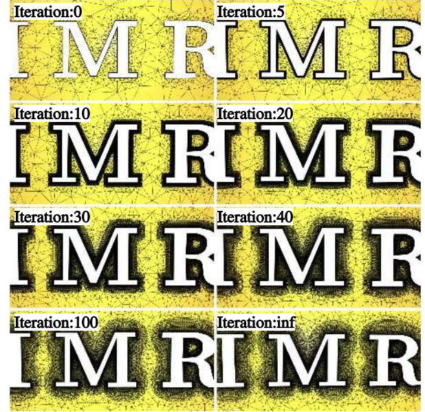
Figure 9: The initial mesh and the air mesh of the IMR English letter model by a different number of iterations.
