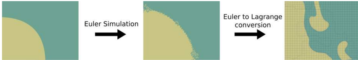
Figure 1: From left to middle, during an hydrodynamic simulation on a grid where two materials are defined (green and yellow) the interfaces between the two materials evolve. For running a Lagrangian code that requires a pure conformal mesh as an input, the mesh must be adapted along with material interfaces. Zoom is performed on the right on the final Lagrangian mesh.
